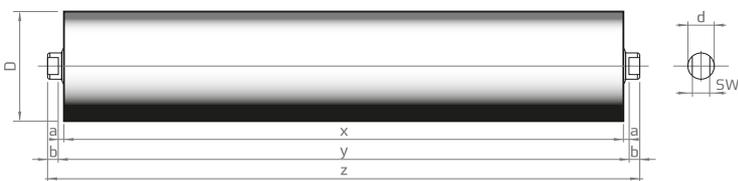
**Primer oznake:** OV valjak tip OV 89-20; x=315; SW 14 / standardne dužine (x) mm valjaka: / **For example:** OV roller type OV 89-20; x=315; SW 14 / standard length (x) mm valjaka:
